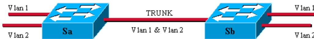
In this diagram, the unique physical link between the two switches is able to carry traffic for whatever VLAN. In order to achieve this, each frame sent on the link is tagged by Sa so that Sb knows to which VLAN it belongs. 802.1Q uses an internal tagging mechanism. Internal means that a tag is inserted within the frame, as shown below.
