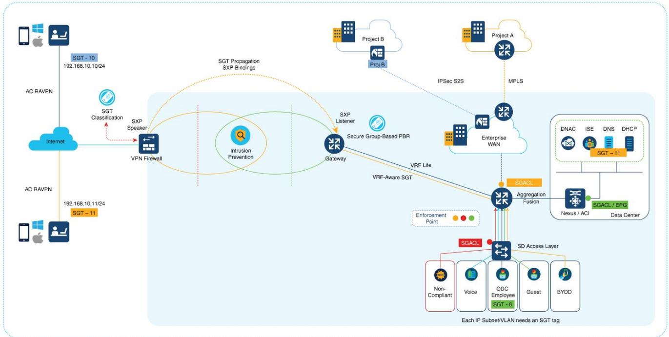
**Note:** ASA can also have SGFW controlling the traffic that comes from a remote VPN user. For example, traffic between a remote VPN user with SGT 10 and SGT 11 can be controlled through SGFW.
