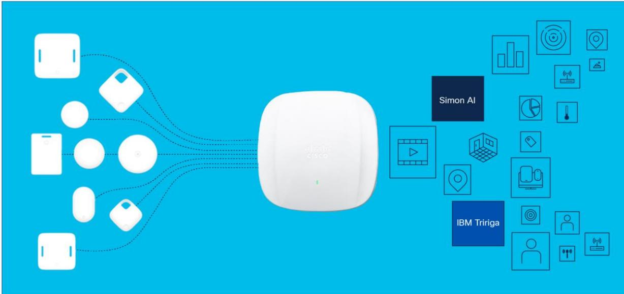
**Figure 22.** Wi-Fi 6 access point gateways enable BLE end devices such as BLE beacons and asset tags
