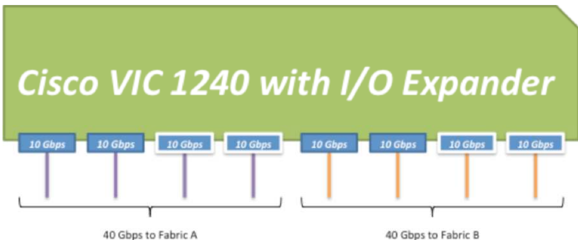
Figure 2. Cisco VIC 1240 with I/O Port Expander
