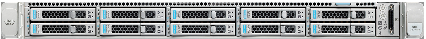
Figure 7. Cisco UCS C225 M8 Rack Server
