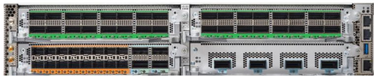
Figure 3. 8712-MOD-M chassis with 4 Modular Port Adapters (8K-MPA-16H on top left and right, 8K-MPA-16Z2D on bottom left, 8K-MPA-4D on bottom right)
