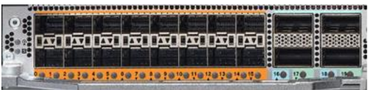
Figure 7. 16 port SFP56 and 4 port QSFP56 DD that can be used as 2x400G or 4x100G/200G
