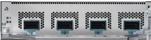
Figure 5. 4 port QSFP56 DD MPA
