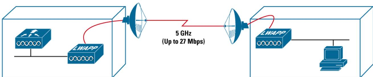
**Point-to-point wireless access with integrated wireless backhaul**—In this application, two bridging access points (Cisco Aironet 1030) are interconnected via a wireless link. One of the bridges is connected to a wired network that has a wireless LAN controller on it, while the remote access point offers service in one band, and uses the other band for backhaul (Figure 2).
