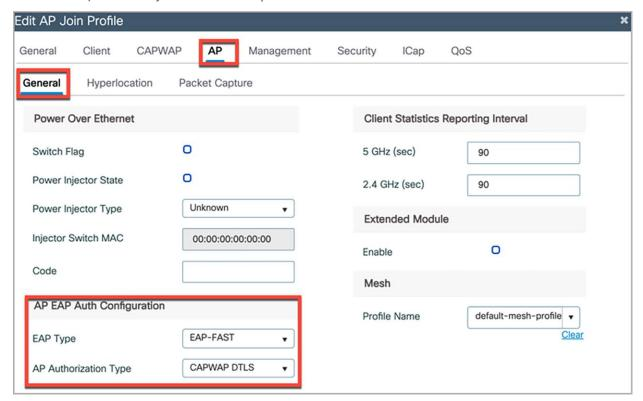
Control and Provisioning of Wireless Access Points (CAPWAP) Datagram TLS (DTLS) LSC support on the access point is used for provisioning and downloading the certificate onto the access point.
