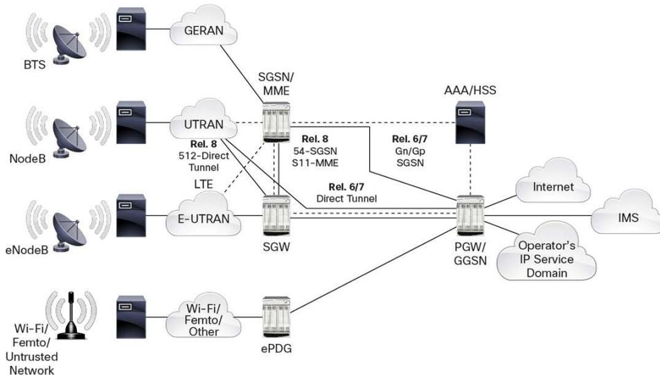
For instance, the MME, SGW, and PGW can be combined into one carrier-class platform. By collapsing these functions, operators could reduce the signaling overhead, distribute session management, and use the control and user plane capabilities of the carrier-class node.
