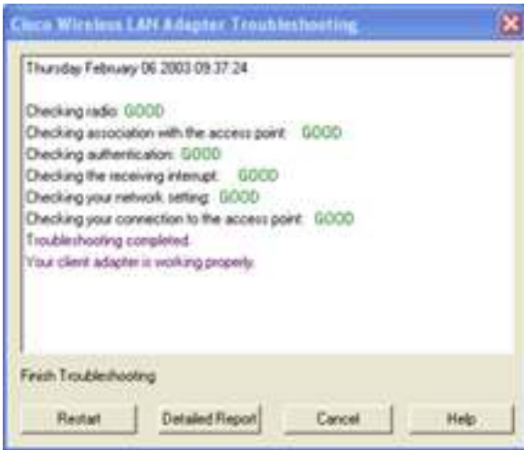
Figure 5. Troubleshooting Facility gives step-by-step details on the process of connecting to an access point.
