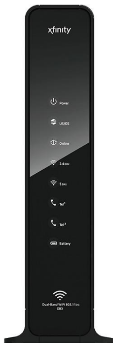
Figure 1. Cisco Model DPC3941B DOCSIS 3.0 24x4 Wireless Business Gateway (Image Below May Vary from Actual Product)
