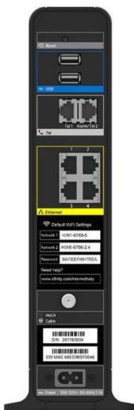
Figure 3. Cisco Model DPC3941B Business Gateway Back Panel (Image Below May Vary from Actual Product)
