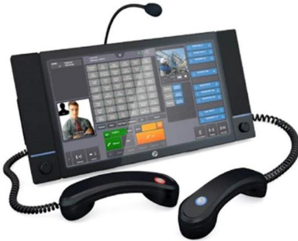
Figure 5. IP Command Touch Screen Dispatch Consoles
