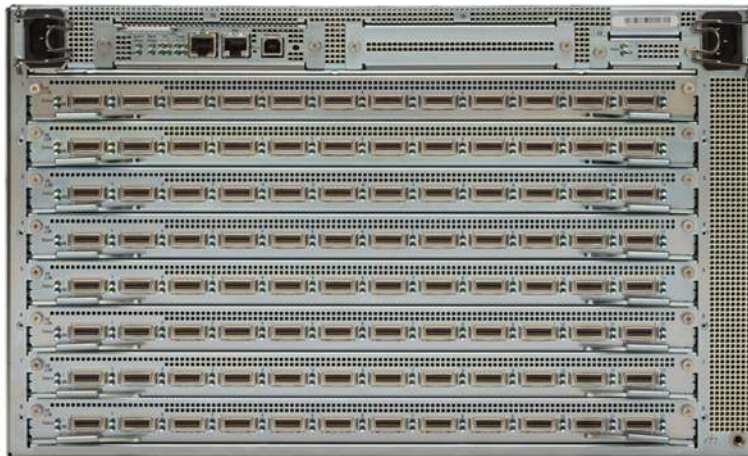
Figure 2. Cisco SFS 7008P Back Side, with Switch Ports and Redundant Power and Management
