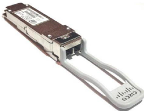
The Cisco QSFP BiDi transceiver has two 20-Gbps channels, each transmitted and received simultaneously over two wavelengths on a single MMF strand. The result is an aggregated duplex 40-Gbps link over a MMF duplex LC-terminated fiber cable. The connection can reach 100 meters on OM3 MMF or 150 meters on OM4 MMF, which is the same as 40-Gbps SR4. Figure 3 shows the technology concept of the Cisco QSFP BiDi transceiver.
