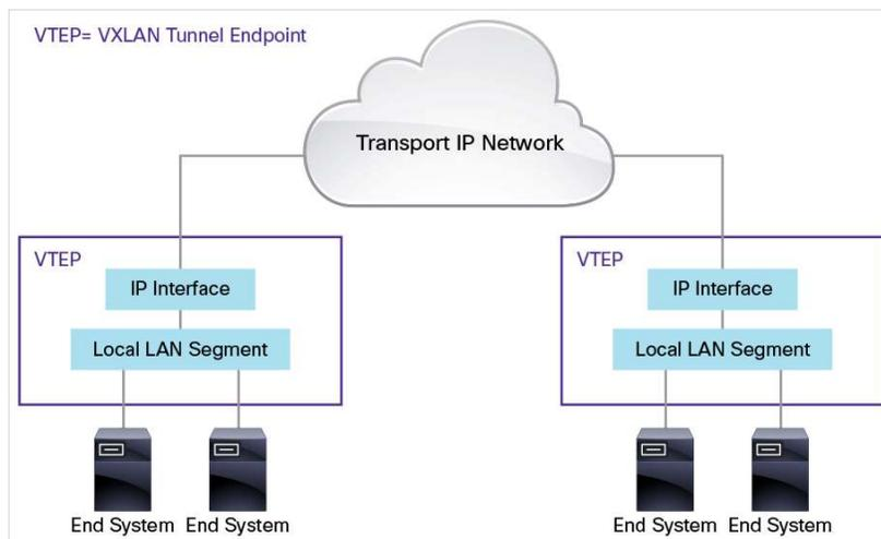
VXLAN is designed to provide the same Ethernet Layer 2 network services as VLAN, but with greater extensibility and flexibility. In comparison to VLAN, VXLAN offers the following benefits:
