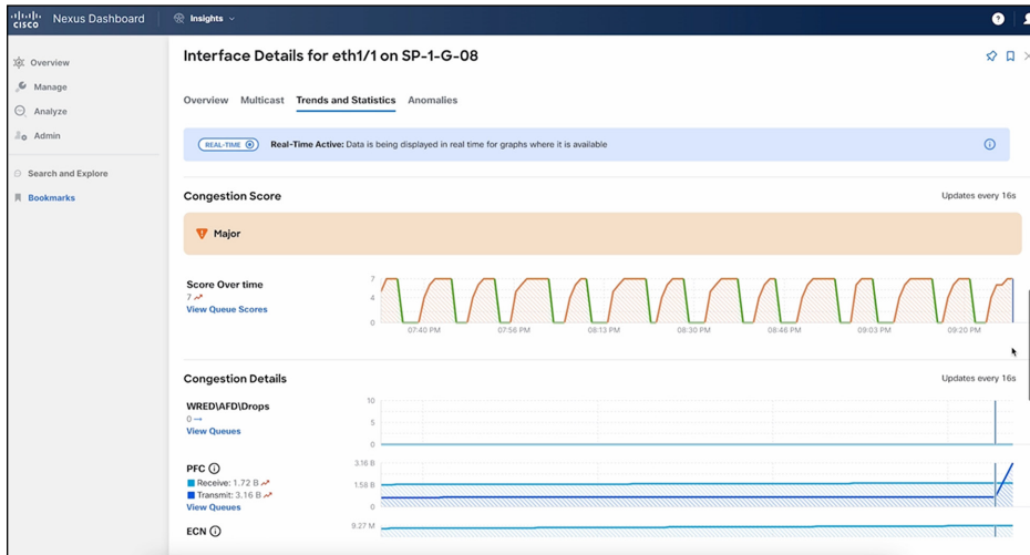
Figure 9. Nexus Dashboard showing congestion score with automatic red, orange, and green categorization
