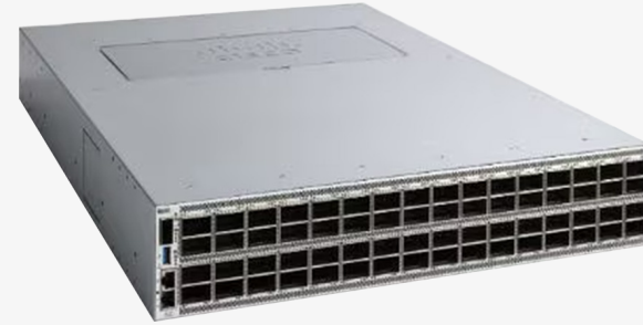
Figure 5. Cisco N9364E-SG2 switch
