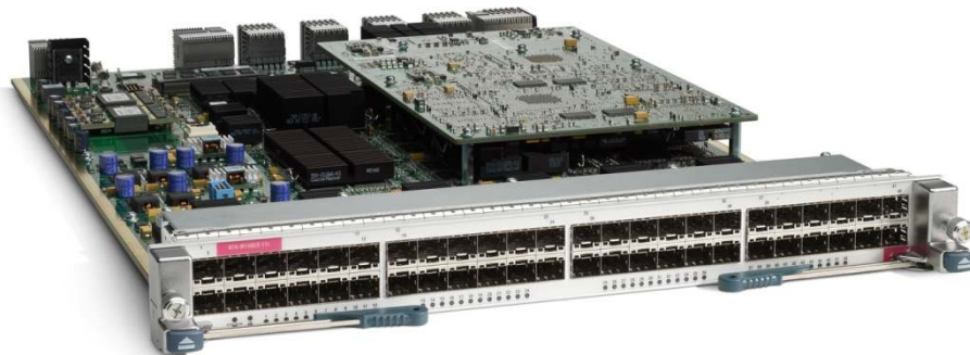
Figure 3. Cisco Nexus 7000 Series 48-Port Gigabit Ethernet Module with XL Option
