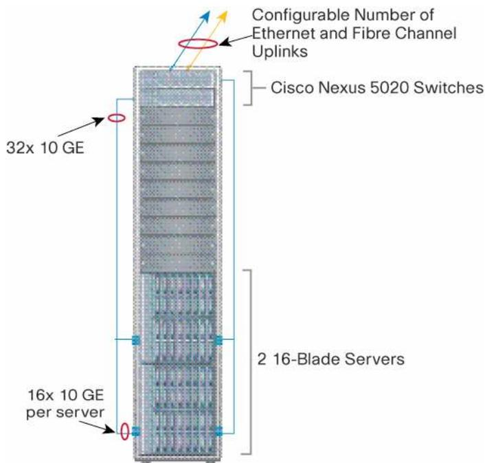
In this example, 32 of the fixed Cisco Nexus 5020 ports on each switch are occupied with network links to blade systems, leaving 8 fixed ports available for network uplinks. This configuration yields an Ethernet network oversubscription ratio of 4:1. Note that this configuration allows full line-rate connectivity between all blades in the rack with no oversubscription in the rack.
