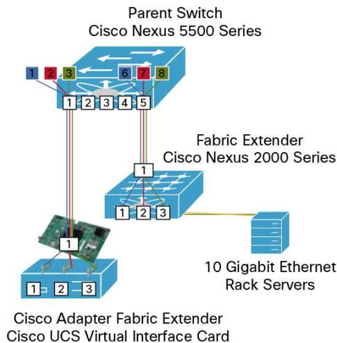
The Cisco Adapter FEX is logically an extension of the parent switch inside the server.
