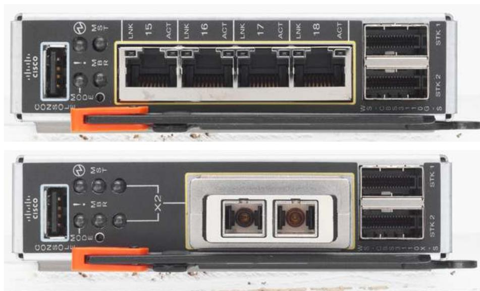
Two products form the CBS3110 family: CBS3110G and CBS3110X. The CBS3110G provides four copper RJ45 based Gigabit Ethernet uplink ports. The CBS3110X has a single 10GE X2 based uplink port. This port supports SR, LRM, CX4 and TwinGig modules. Future support for LR and LX4 modules will be provided post FCS.
