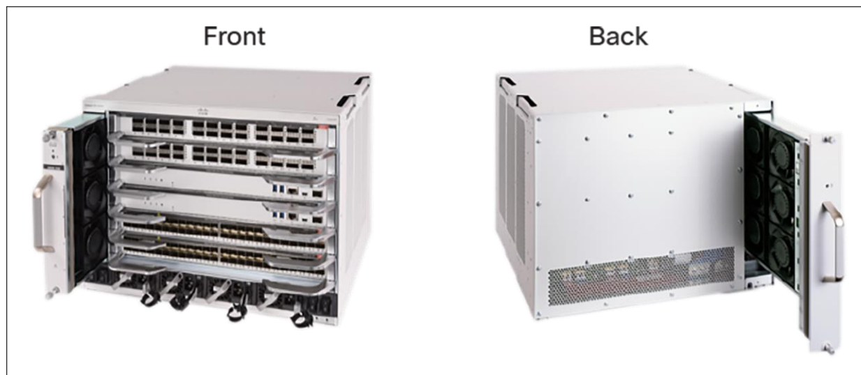
Figure 5. Flexible fan-tray servicing
