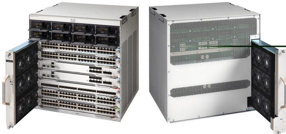
Figure 2. Dual serviceable fan tray
