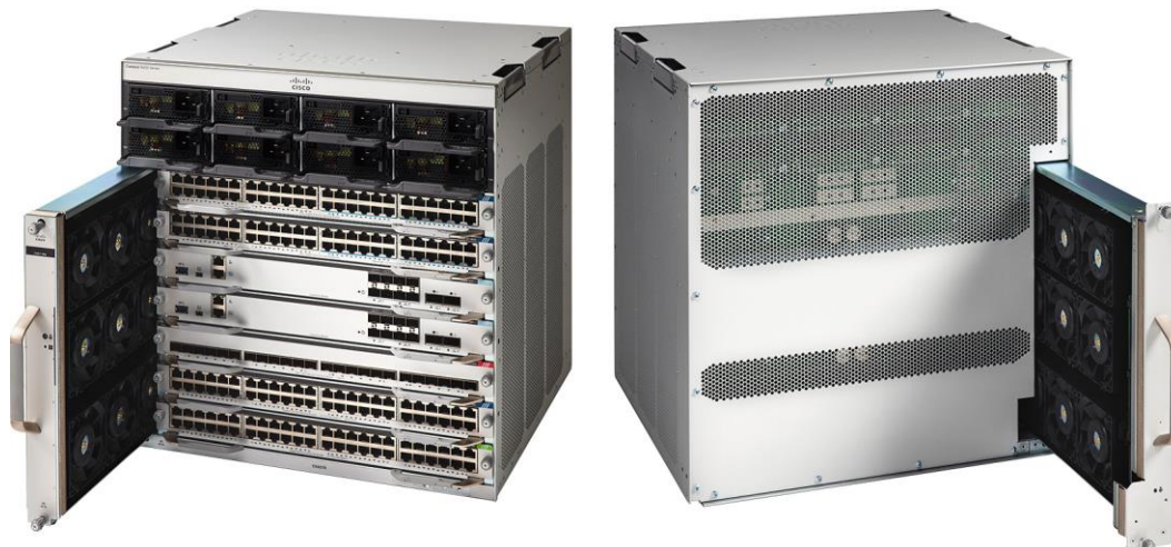
Figure 2. Dual serviceable fan tray
