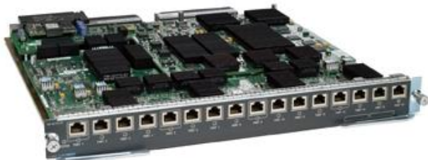
Figure 1. Cisco Catalyst 6500 16-Port 10 Gigabit Ethernet Copper Module
