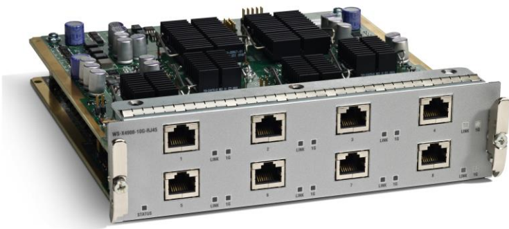
Figure 2. Cisco 8-Port (2:1) 10GBASE-T (RJ-45) Half-Card
