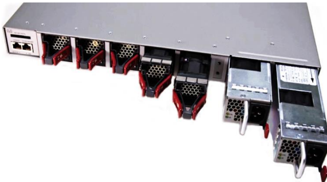
Figure 6. Redundant Fan and Power Supply
