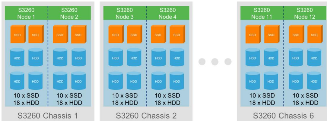
Figure 7. Logical Design Example for Cisco UCS S3260 for an IOPS-Intensive Object Storage Solution
