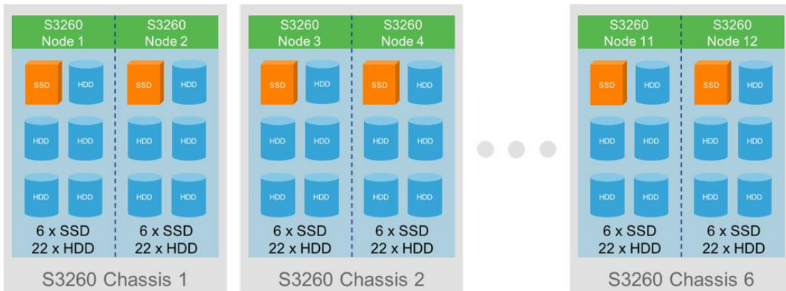
Figure 8. Logical Design Example for Cisco UCS S3260 for a Throughput-Intensive Object Storage Solution
