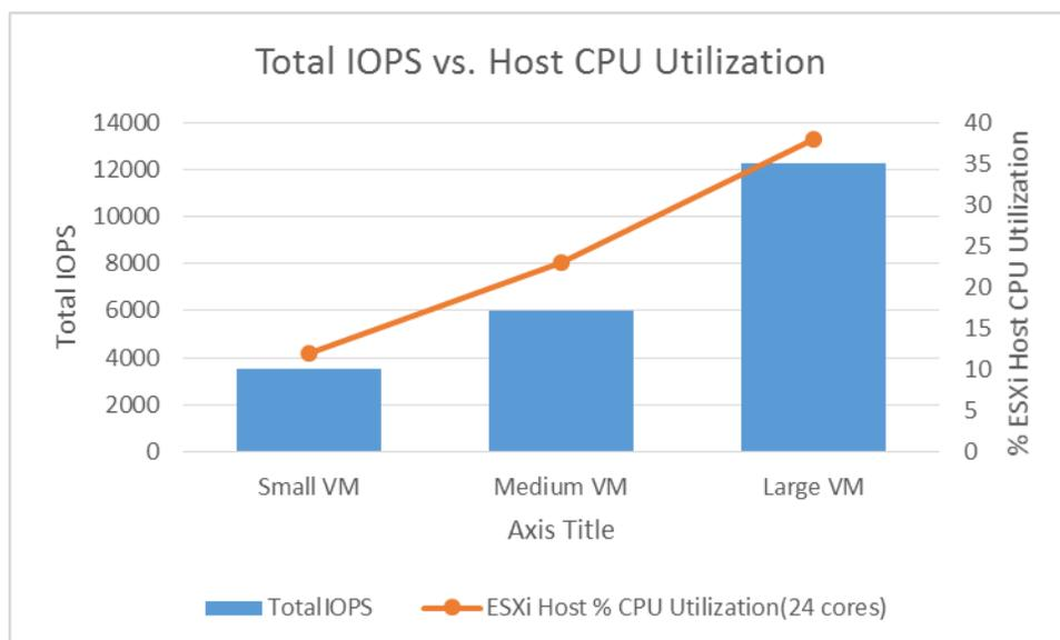
It is clear that the IOPS scale linearly with the size of the VM, and CPU utilization per VM is calibrated at roughly 12 percent of the total available physical CPU for the small VM tile. This is the baseline VM characterization for the scaling study, and is not to be confused with the system capabilities.
