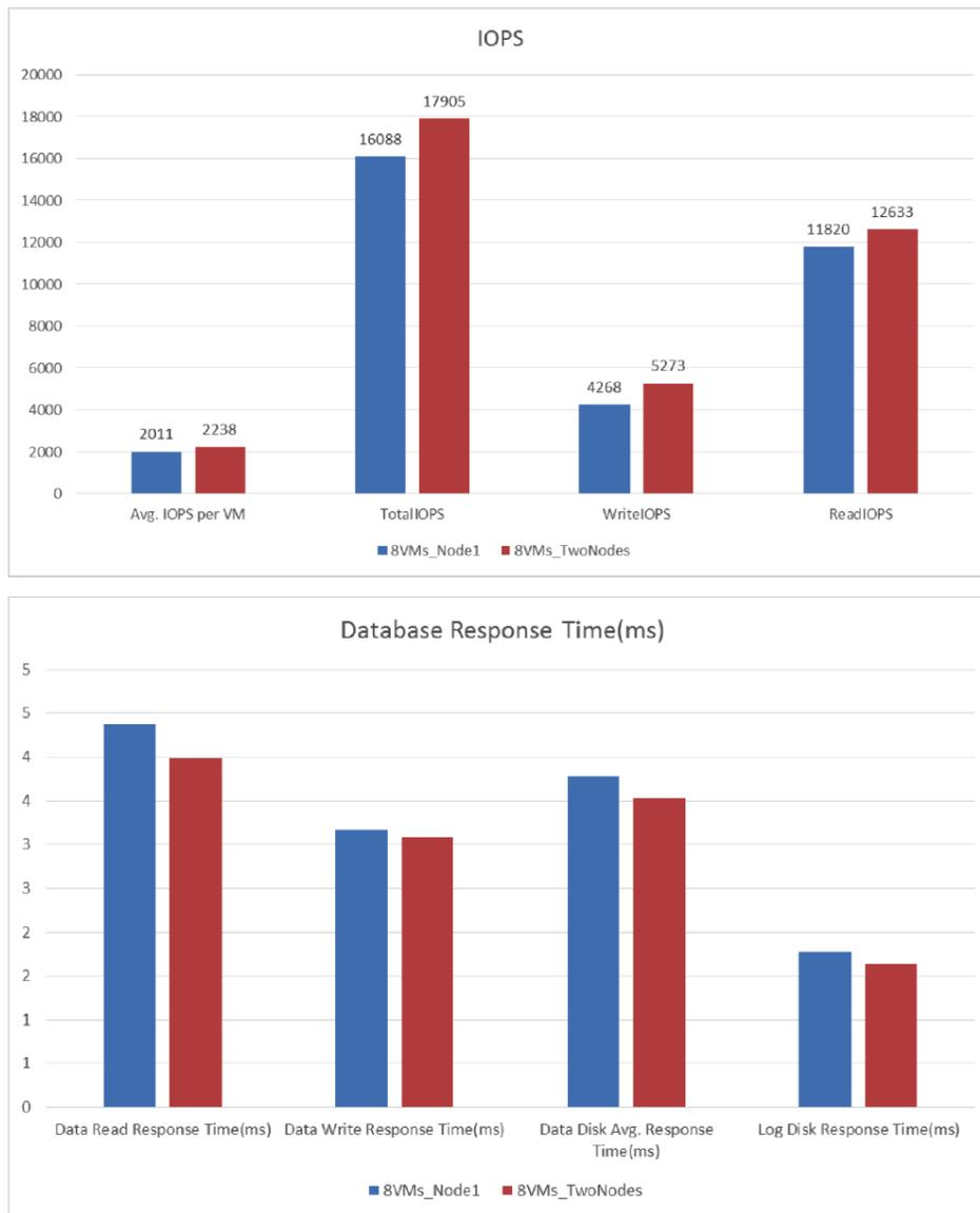
There was not much noticeable degradation between the steady state and failure state after the failover of the VMs to the survival node. Both IOPS and response time for the log and data were within acceptable limits.
