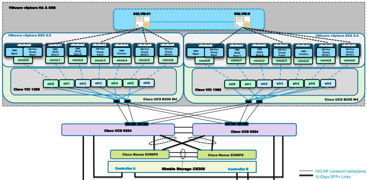
Each vSwitch has a virtual network interface card (vNIC) carved out on Cisco UCS Virtual Interface Card 1380, which serves as an uplink to the Cisco UCS 6324 Fabric Interconnect. It is important to note that vNICs supporting the iSCSI traffic are not configured for automatic failover at the Cisco UCS Manager. HA for the iSCSI traffic is taken care of at the iSCSI initiators level.
