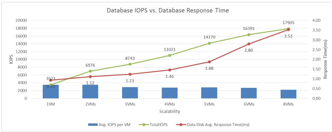
The scale testing of small VM tiles was done by scaling from one to eight VMs, using CS300 as the storage back end. With up to five VMs, the test was run on a single blade, and with six and eight VMs, it was equally distributed between two blades. As you can see, the system scales well up to eight VMs while keeping the response time well within 5 milliseconds (ms) for the average disk I/O operations.
