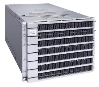
The server offers a choice of 8 NVIDIA HGX H100 or H200 Tensor Core GPUs, or 8 AMD MI300X and MI350X OAM GPUs to deliver massive, accelerated computational performance in a single server, as well as one NVIDIA ConnectX-7 NIC or NVIDIA BlueField-3 SuperNIC per GPU to scale AI model training across a cluster of dense GPU servers.
