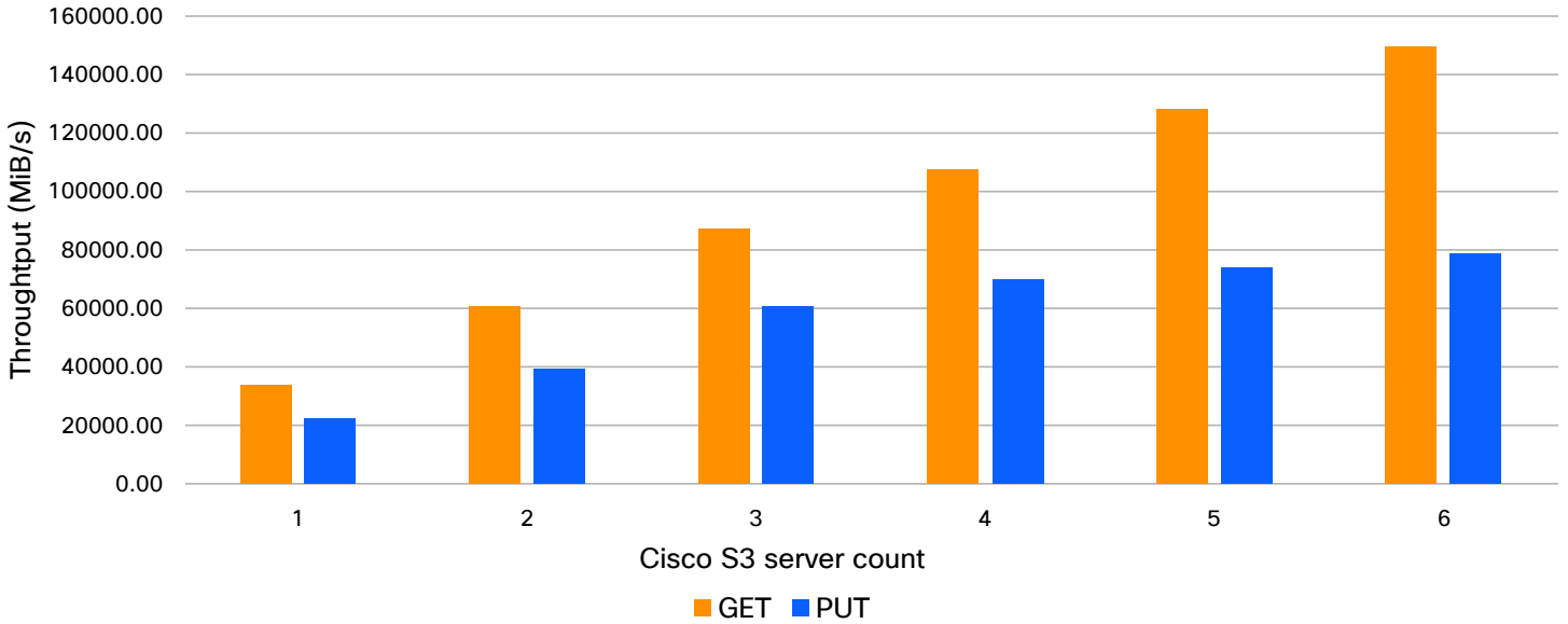
Figure 5. DDN Infinia S3 throughput performance scaling
