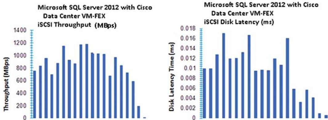
Comparison of iSCSI Network Throughput and Disk Latency with Cisco Data Center VM-FEX and VMware vSwitch
