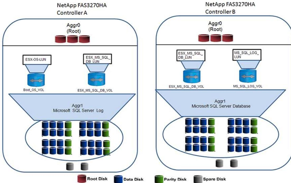
The NetApp iSCSI target was configured with virtual interface-enabled multimode (Link Aggregation Control Protocol [LACP]) cluster failover on each NetApp controller over dual 10 Gigabit Ethernet interfaces, which were part of the Cisco Nexus 5548UP vPC domain.
