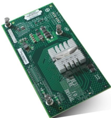
Figure 1. Cisco UCS CNA M61KR-I Intel Converged Network Adapter
