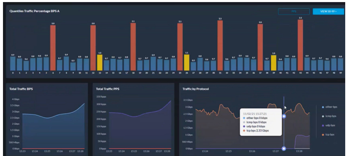
Figure 16. Quantiles – visualization of an attack with attack traffic against legitimate traffic
