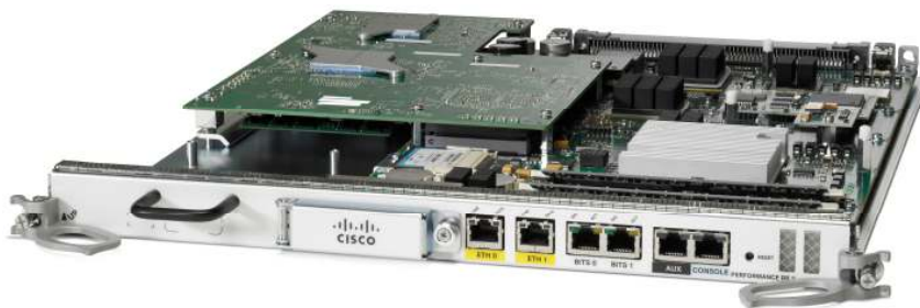
Figure 2. Cisco XR 12000 PRP-3 with PRP3-SMDC Inserted
