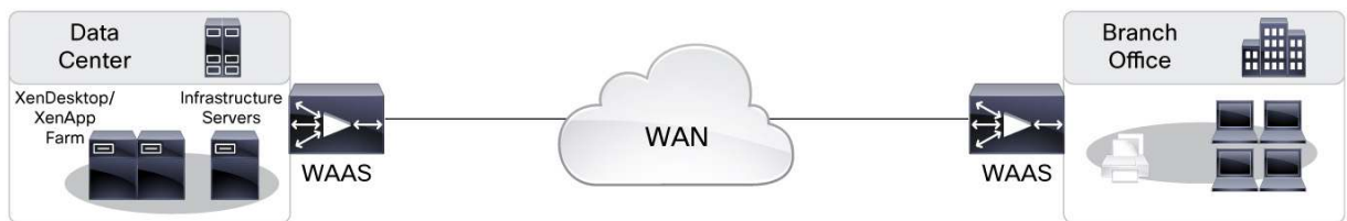
Figure 1. Cisco Optimization for XenDesktop Solution Components
