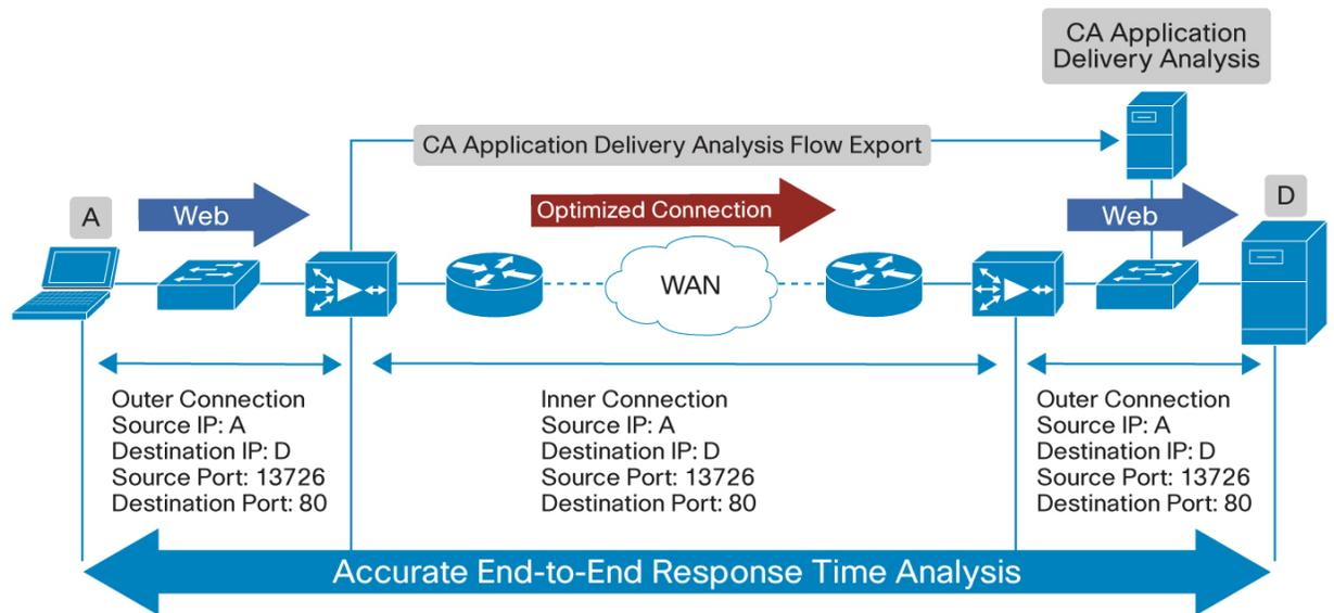
The integration between Cisco WAAS and CA Application Delivery Analysis offers a solution that can accurately measure performance of crucial metrics in specific segments such as the LAN (outer connection A or D), WAN (inner connections), and server (outer connection D) sides. The remainder of this document examines some of the main graphs.
