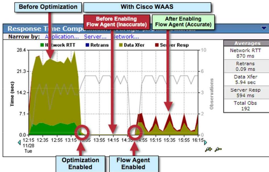
Figure 6 shows how Cisco WAAS optimizations improved application performance and WAN utilization efficiency. By improving efficiency, Cisco WAAS can alleviate congestion encountered on the network, thereby reducing the perceived RTT encountered on the WAN caused by congested router queues and inefficient bandwidth consumption.
