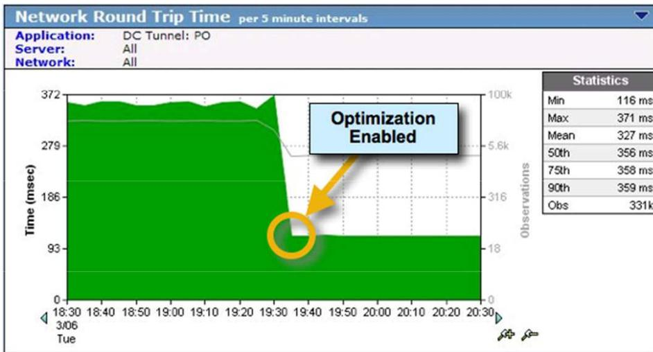
The CA NetQoS Performance Center allows reporting through a single console for both CA Application Delivery Analysis and the Cisco WAAS Central Manager (Figure 7). This complementary capability provides an exclusive integrated solution for understanding the effect of WAN traffic optimization on bandwidth reduction and true end-user experience. From a single dashboard report, you can:
