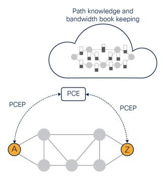
Figure 3. PCE for path computation and bandwidth tracking
