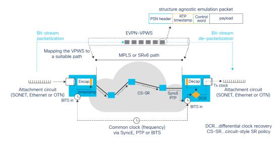
**Figure 2.** PLE operates at the bit-stream level
