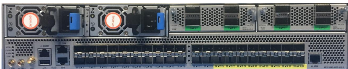
Figure 1. The Cisco NCS-55A2-MOD Chassis
