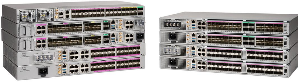
Figure 1. Cisco NCS 540 Medium Density Router Family
