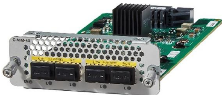
Figure 2. C-NIM-4X: Cisco 4-port 1G/10G LAN/WAN NIM with IEEE 802.1AE MACsec
