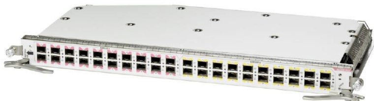
Figure 1. Cisco CRS 40x10 Gigabit Ethernet Interface Module
