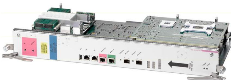
Figure 2. Cisco CRS 16-Slot Line Card Chassis Performance Route Processor
