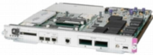
Figure 1. The Cisco 7600 Route Switch Processor 720 with 10 Gigabit Ethernet Uplinks
