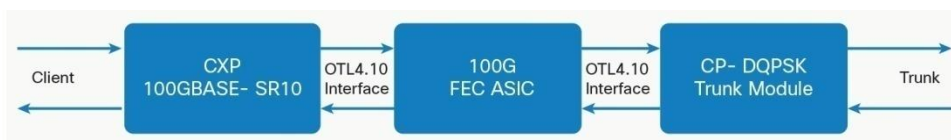
Figure 2. 100-Gbps Full-Band Tunable CP-DQPSK Transponder Card Block Diagram
