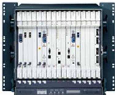
Figure 1. Cisco ONS 15454 ANSI/SONET System
