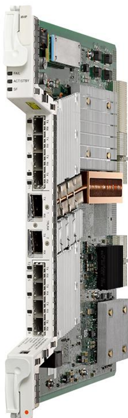
Figure 1. Cisco ONS 15454 Any Rate Enhanced XPonder Card
