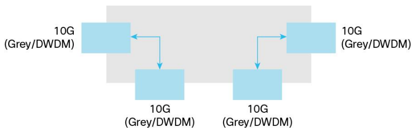
Figure 2. Cisco ONS 15454 OTU2 XPonder Card Logical Scheme
