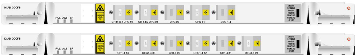
Figure 1. 16-Port (Top) and 12-Port (Bottom) Cisco NCS 2000 Contentionless Add/Drop Line Cards
