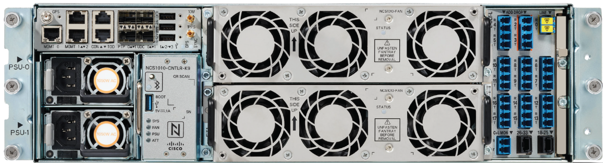
Figure 14. NCS 1010 OLT-L with LC ports on faceplate (L-Band)
